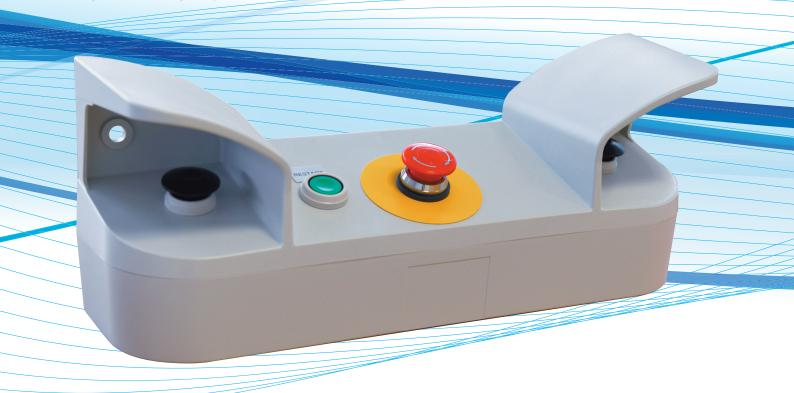
When the two buttons are pressed simultaneously a pneumatic signal is present at the output. As soon as one or both buttons are released the signal will be lost. The two-hand control panel is additionally equipped with an emergency stop button for venting in case of emergency. The restart function eliminates potential hazards due to energy failure and energy recovery.
